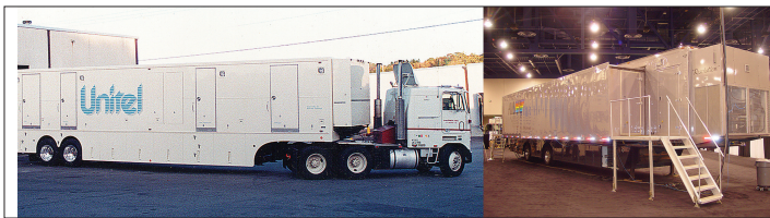
Figure 8.14 High-end trucks continue to push the limits of technology. The truck on the left was state of the art in the 1980s; the one on the right is on technology's edge today. The new truck is All Mobile Video's truck named "Resolution." This is a high-definition (HD) truck that can handle up to 16 cameras and 20 VTRs. This truck is a hybrid, in that it can produce both HD and SD outputs at the same time. Up until recently shows that were offered in both SD and HD used two separate production units and crews. Panasonic built a truck and lent it to ABC for a year of Monday Night Football, and CBS has hired SWTV and others to cover a few NFL and college football games, most separately from the SD feed. Other early HD trucks have been put into service by NMT, AESM and HD Vision. Airing simultaneous SD and HD productions presents problems other than the technical ones. The production techniques used for HD are often different. The increased resolution that HD offers allows for wider shots, capturing more of the overall spectacle, and HD has a wider aspect ratio, 16:9 vs. SD's 4:3. The HD cameraman has to keep in mind that he must keep the entire pertinent scene in a narrower 4:3 box for SD viewers, but at the same time keep unwanted people and things out of the HD viewer's picture.
